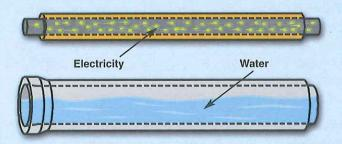
With Snap Circuits the wires you will use have been shaped into snap wire strips, to make interconnection easy. These work the same as any other wires you might find in your house, since they are made of metal.
